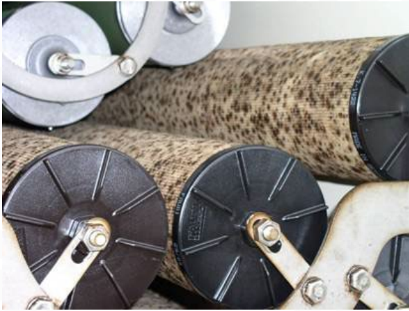
Leopard spotting / fungal growth on Filter Water Separator coalescer elements (EI 1581)
