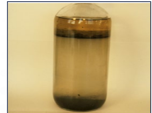
Black/grey discolouration of water and fuel due to sulphide generation by SRB
