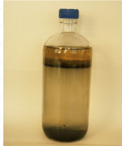
Black/grey discolouration of water and fuel in tank bottoms due to sulphide generation by Sulphate Reducing Bacteria (SRB)
