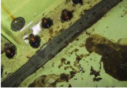
Floating Interface Biofilm (Type I)
