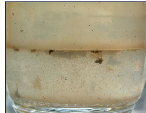
Hazy fuel due to microbial biosurfactants emulsifying water in fuel
