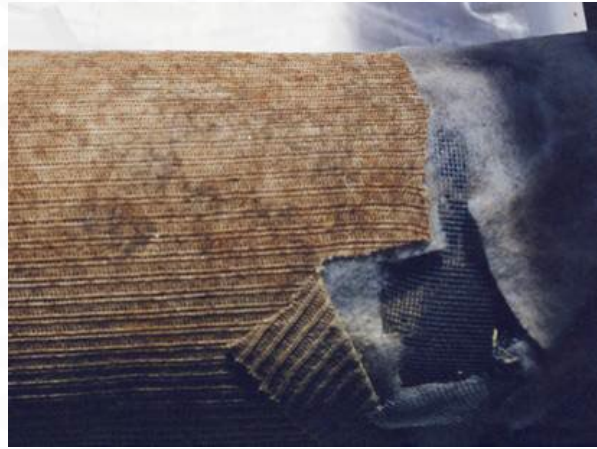
Leopard spotting / fungal growth on Filter Water Separator coalescer elements (EI 1581)
