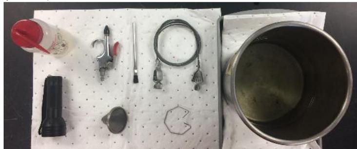
Equipment for hose-end strainer cleaning procedure.
