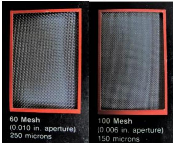
(Hose-end strainers 60mesh vs 100mesh):
