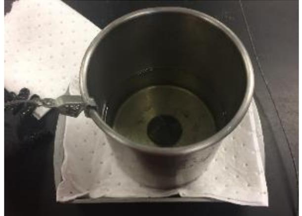
After agitating the hose-end strainer in fuel as described above, at least one of the below procedures shall be followed to complete the cleaning process. In any case, regardless of the option chosen, rinse the strainer in fresh fuel before returning the strainer to service.
